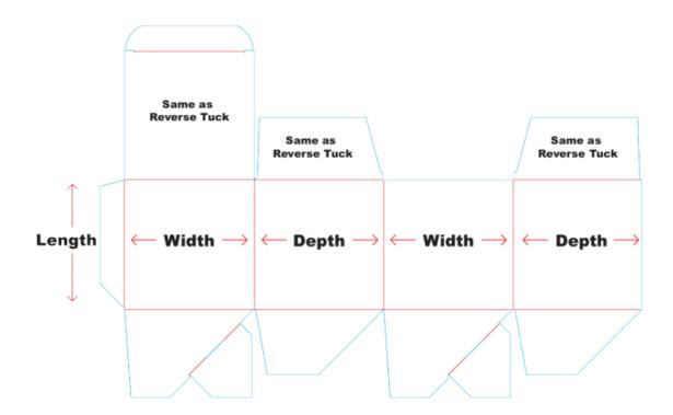
Check for errors: Double-check the dieline for errors such as incorrect measurements, missing or incomplete information, or overlapping lines.
